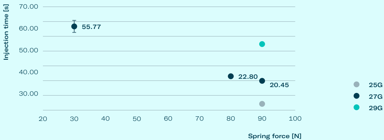
Figure 4 Injection times of 3 mL of 1 cP liquid (water) at three different force levels using the Gx Inbeneo® platform simulator.
